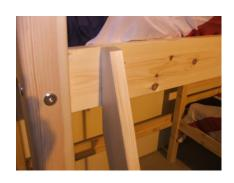
Line the ladder up so it sits level, again using the black screw fix from the inside into the ladder. There are no pilot holes as each bed will have this positioned different given the floor level.
